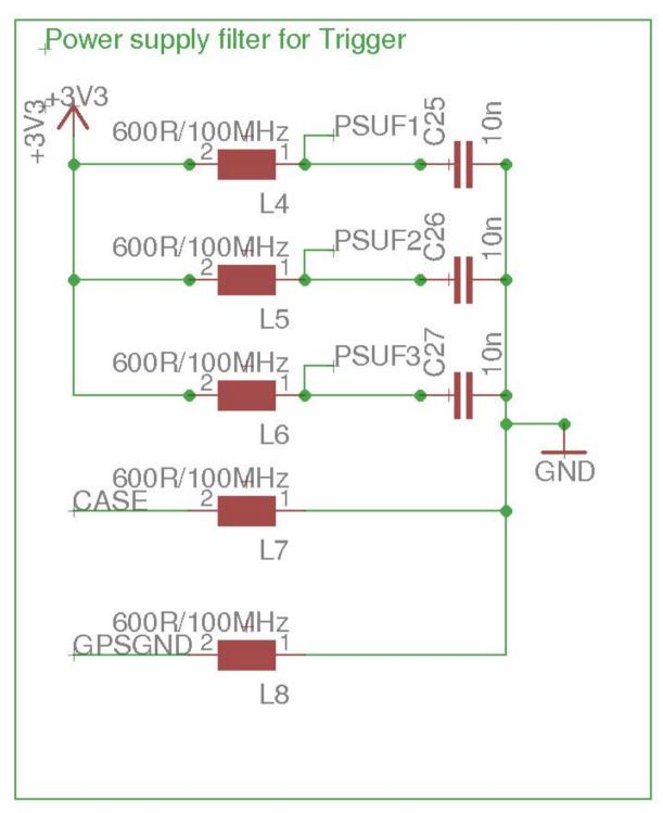
The power supply filter block uses ferrite beads (surface mount 600R/100MHz) to prevent high frequency noise transmission between the functional blocks.
