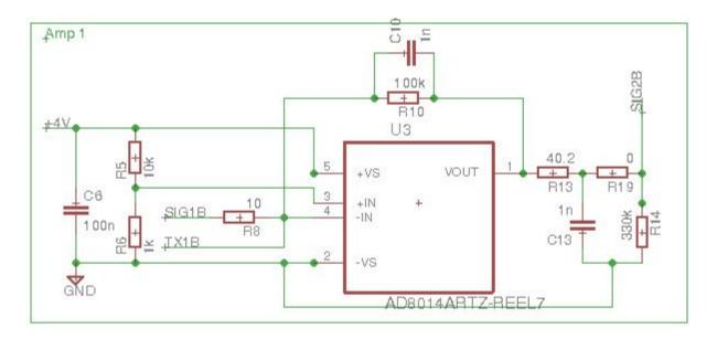
Figure 5: Amplification and shaping stage
