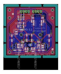
Figure 1: Analogue Board Version 2.2 (2.3 is the same just with 0806 LEDs)
