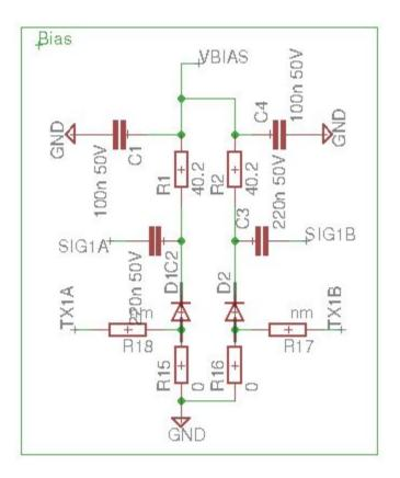
Figure 3: Bias configuration for SiPMs
