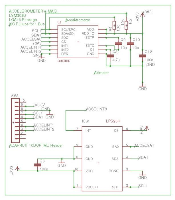
The Inertial Measurement Unit (IMU) is comprised of two discrete IC's which replicate the functionality of the Adafruit 10DOF IMU header. A 10 pin 2.54mm pitch
