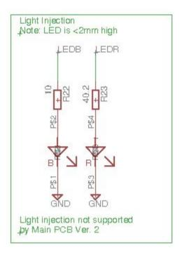
Figure 7: LEDs for Light Injection
