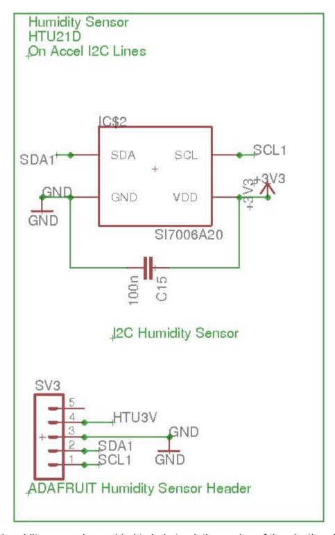
A humidity sensor is provided to help track the ageing of the plastic scintillator. There are numerous papers which indicate that the presence of humidity has a negative effect on the lifetime performance of certain types of scintillator medium, therefore a sensor has been included to assist in checking the quality of the environment within
